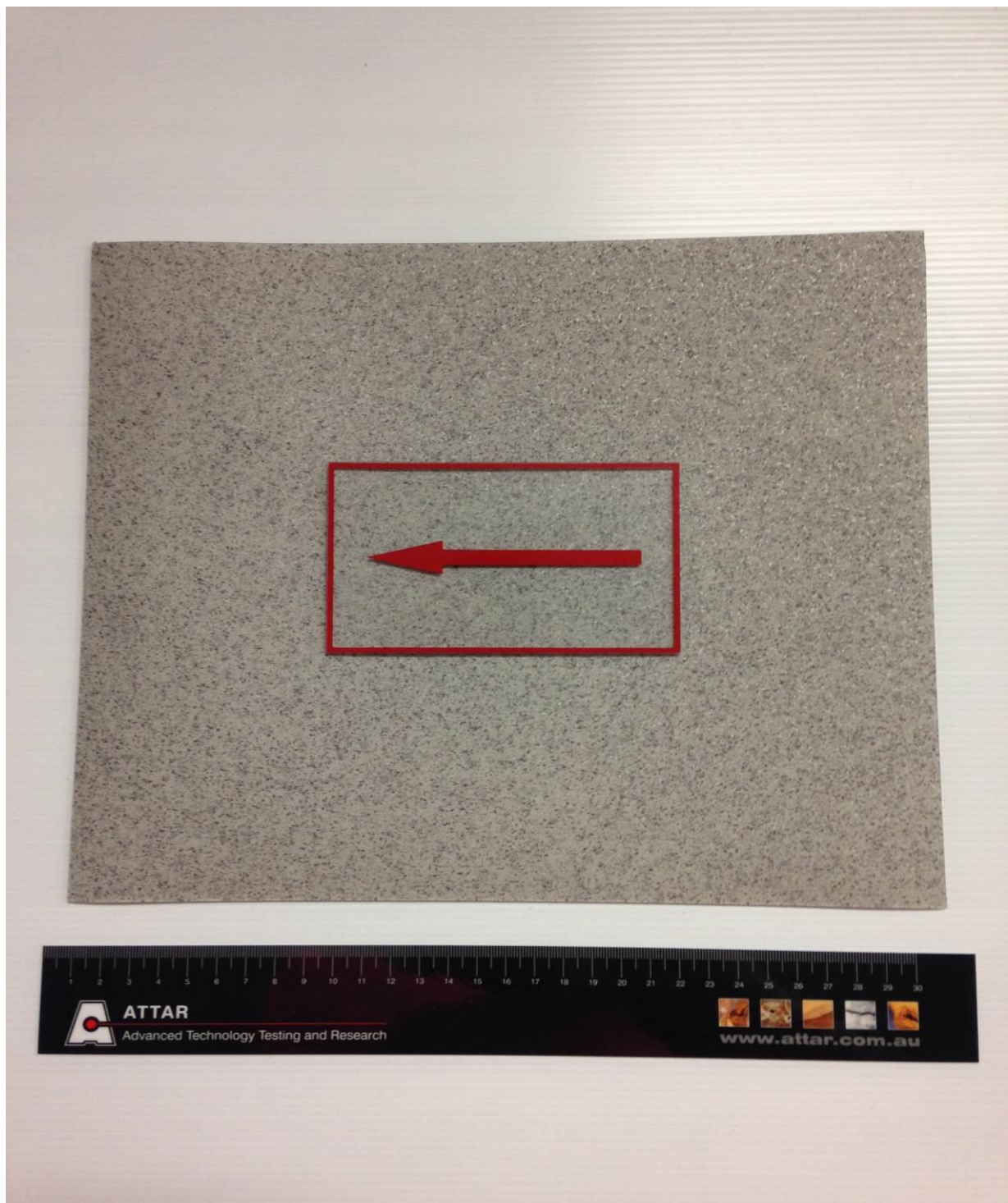
Figure 1: Acczent Ruby – Highlighted area indicates area tested and direction of test.
