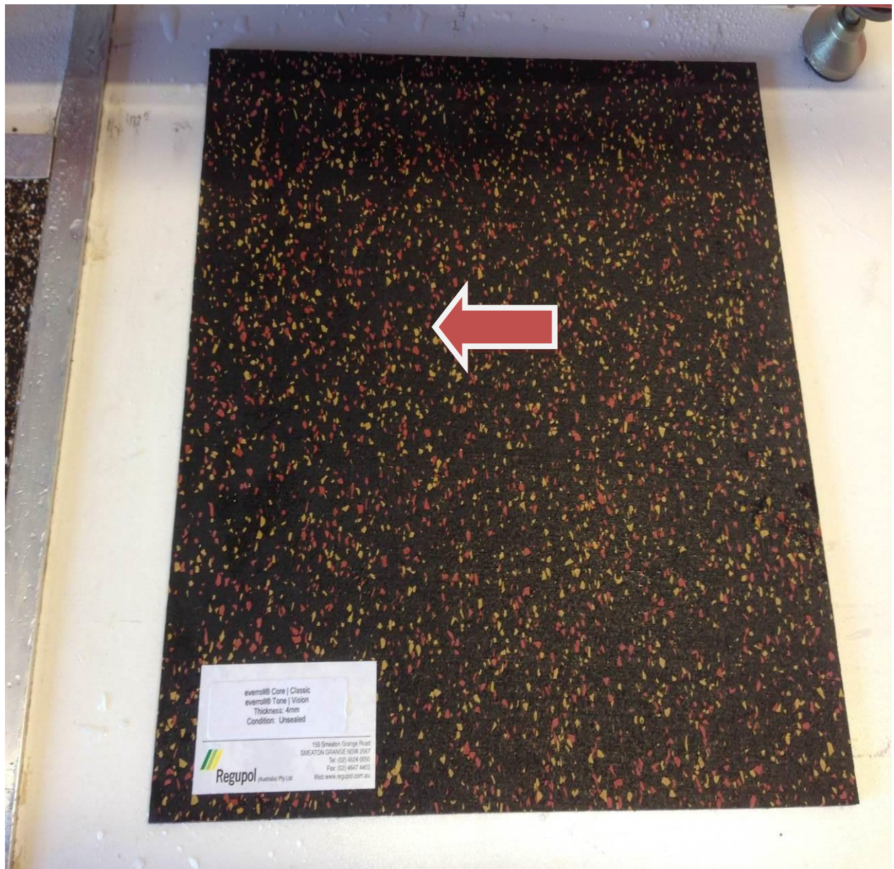
Figure 1: everroll® Core | Classic & Tone | Vision – Highlighted area indicates area tested and direction of test.
