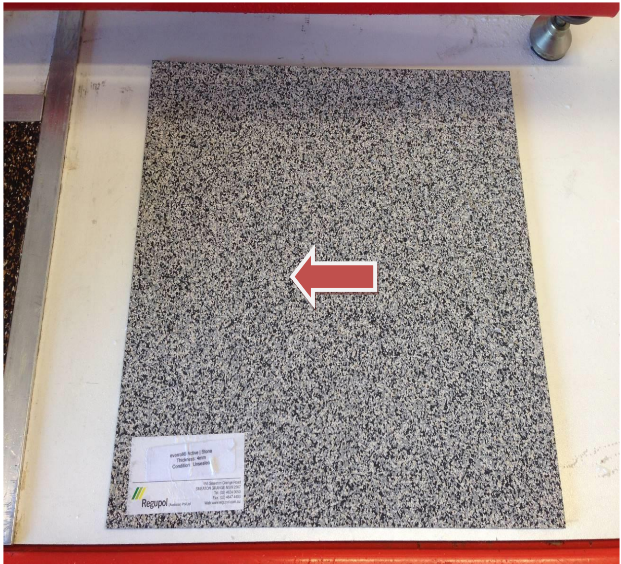
Figure 1: everroll® Active I Stone – Highlighted area indicates area tested and direction of test.
