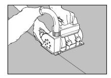
The sheets are heat welded. Do not weld until the adhesive has bonded completely. The joints are chamfered or grooved to about ¾ of the thickness using a hand grooving tool or machine prior to welding. Extra special care must be taken so that copper strips not are damaged during chamfering /grooving.
